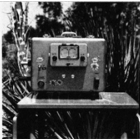
Fig. 11. The d.c. galvanometer and packaged electronic device for testing the amplexus response of young green anoles. The plant shown in the lead photo indicates size.
