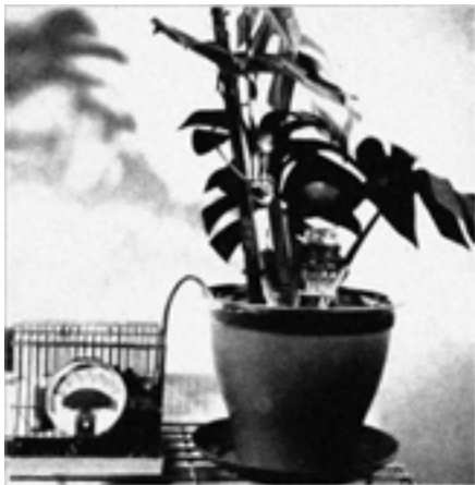
Fig. 8. Indoor arrangement for testing Barkley Effect. The d.c. amplifier is on left, connected by shielded line to the leaf and set-up potentiometer. Nutrient feeder is in the pot.
